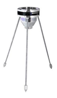
Viscosity Flow Cup NOVOTEST VZ is designed for rapid determination of the relative viscosity (flow time) paints and other related products (Newtonian liquids).
