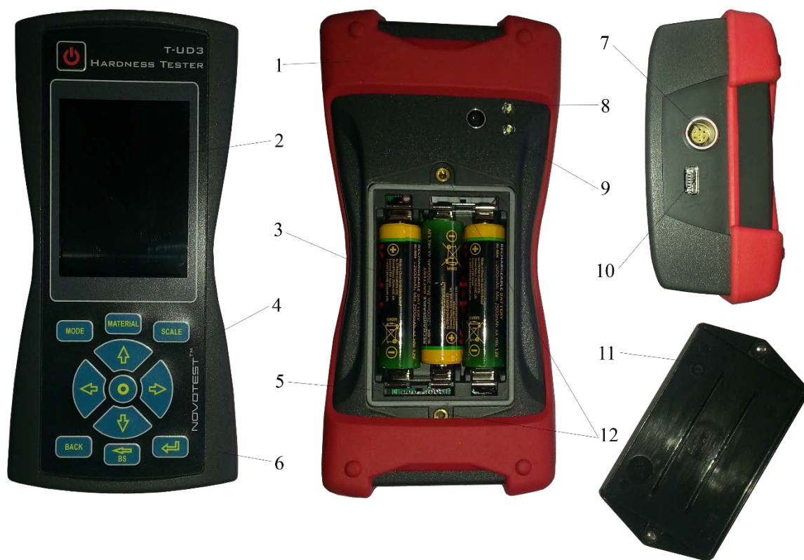
1 – bumper; 2 – LCD/TFT color contrast display; 3 – NiMH battery; 4 – control keyboard; 5 – battery compartment; 6 – electronic unit; 7 – probe socket; 8 – flash light; 9 – photo camera; 10 – mini USB socket; 11 – cover; 12 – threaded connections for cover.
