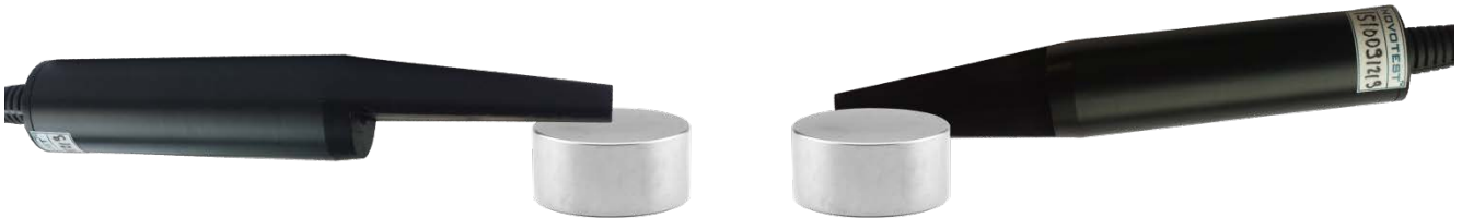
Figure 2.12 – Measurement of the normal component of the induction vector of a constant magnetic field on the end and side surface of the test object
