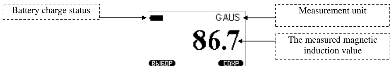
Figure 2.7 – Displaying of information during the operation
