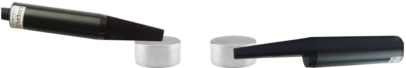
Figure 2.13 – Measurement of the tangential component of the magnetic field induction vector on the end and side surfaces of the test object
