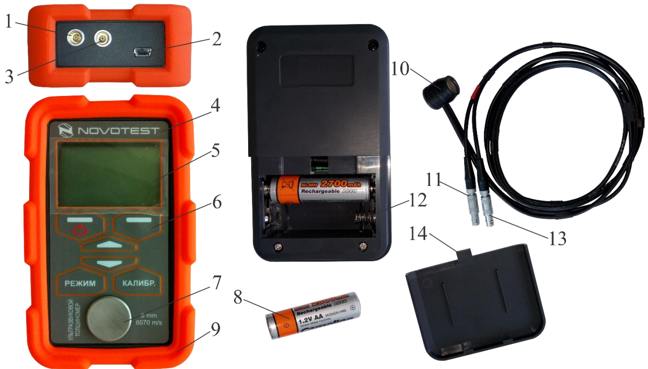
1 - generator socket; 2 – mini-USB connector; 3 - receiver socket; 4 - electronic block; 5 - graphic indicator; 6 - keyboard; 7 - reference sample; 8 – battery storage; 9 - protective silicone bumper; 10 - transducer; 11 - generator plug; 12 - battery compartment; 13 - receiver plug; 14 - battery compartment cover.
