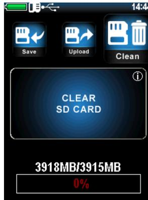
Clearing saved records in the archive and backup copies of calibrations: after clearing SD card the archive will be empty and backup copies of calibrations delete. To clean just stored archival records - transmit saved measurements to PC with special software. Thus backup calibrations will be unaffected.
