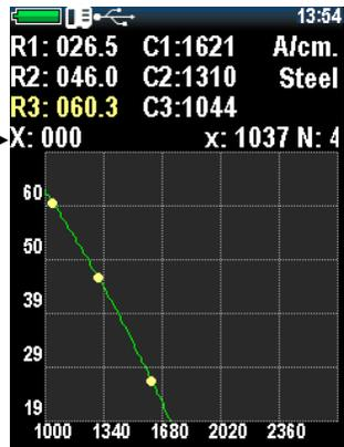
To check the correctness of the got values, move the cursor to the **X:000** and take a few measurements on one of the sample.
