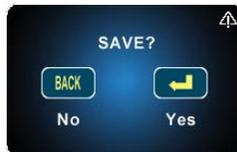
Press **YES** by **RIGHT**. Calibration is saved. Select the appropriate material and scale, and device is ready for operation.
