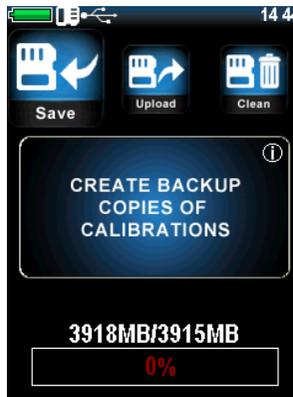
After calibration of the probe is recommended to create a backup copy of the calibration (usually the manufacturer makes the calibration of 1-2 scales, to check the probe). This is done in order to
