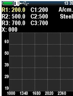
The device, making the measurement, gets the nominal codes, the purpose of calibration - is to find the correlation between the nominal code and coercive force (construction of the relation function).
