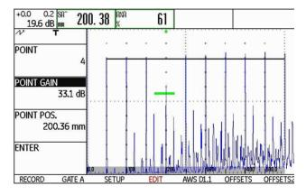
Select the function **POINT POS.** and press the function keys to change the distance of the point.
