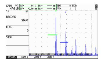
Next to the A-scan, the control functions are displayed in the function group **RECORD**, whereas the settings for each gate in question are displayed in the function groups of gates.
