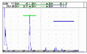
The gain and the adjusted dB step value are shown in the top left corner of the display screen. The access to all other instrument functions is disabled in the zoom mode of the A-scan display.
