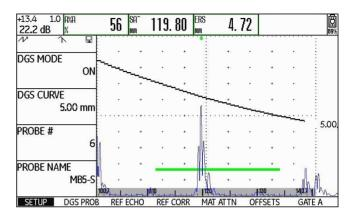
Taking the general DGS diagram as a basis, the USM Go calculates the required test sensitivity for displaying the 3 mm curve with its maximum at 80 % screen height, and makes this setting. The current gain is set to 0 during this.
