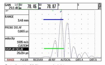
**Gate A** set to 20 % screen height measured sound path **SA/** = 78.46 mm
