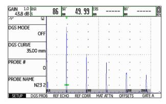
Select the individual functions in the different function groups, and press the function keys to define the corresponding settings: DGS CURVE (recording curve for DGS evaluation)
