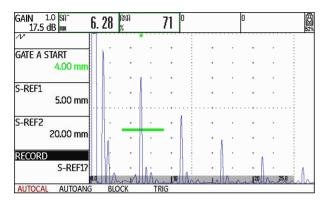
Position the gate on the second calibration echo and record the second calibration echo.
